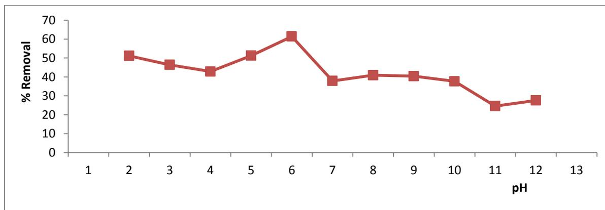
**Fig. 2: A Plot of removal efficiency against initial solution pH**
