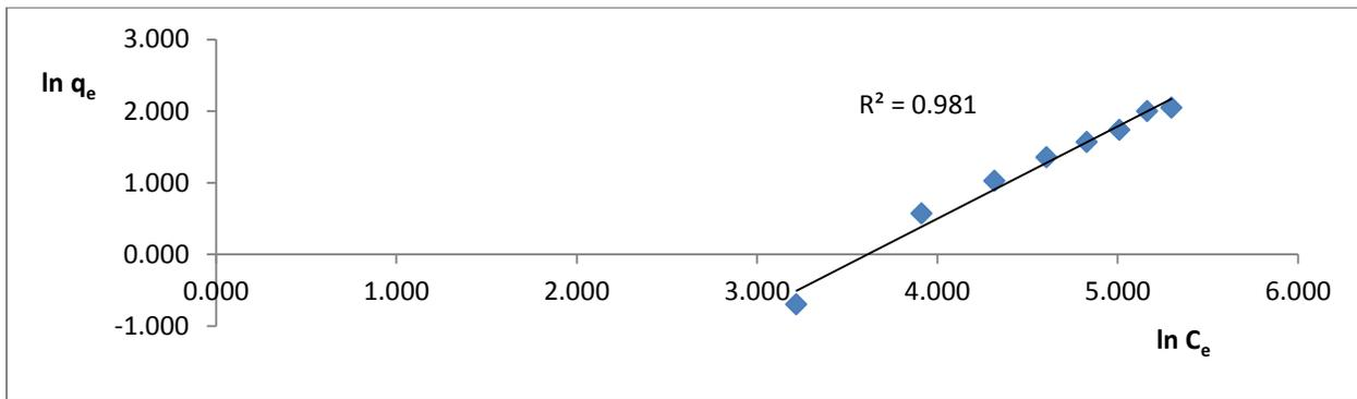
Fig. 9: Freundlich isotherm for Congo red adsorption on Bambara groundnut hull
