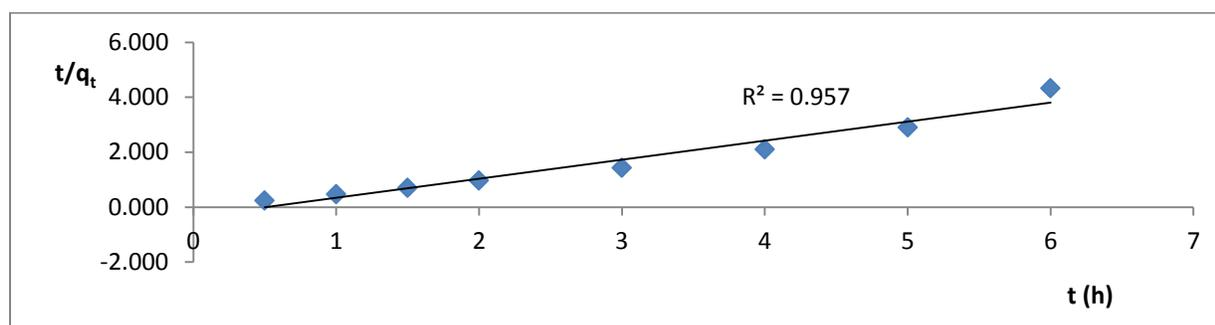
Fig. 7: Pseudo-second order plot for Congo red adsorption on Bambara groundnut hull
