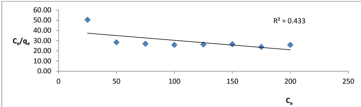
Fig. 8: Langmuir isotherm for Congo red adsorption on Bambara groundnut hull
