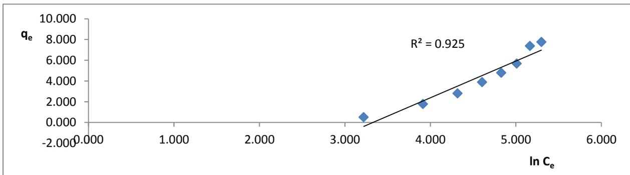
Fig. 10: Tempkin isotherm for Congo red adsorption on Bambara groundnut hull
