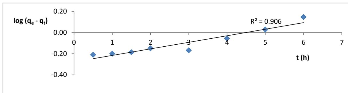
Fig. 6: Pseudo-first order plot for Congo red adsorption on Bambara groundnut hull
